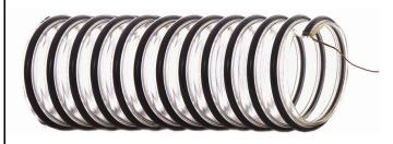
The Model TD11 is a static dissipative polyurethane hose reinforced with a ridgid ABS helix and has an embedded copper grounding wire and smooth interior. This is a hose that can has gread abrasion resistance, but remains extremely flexible.
